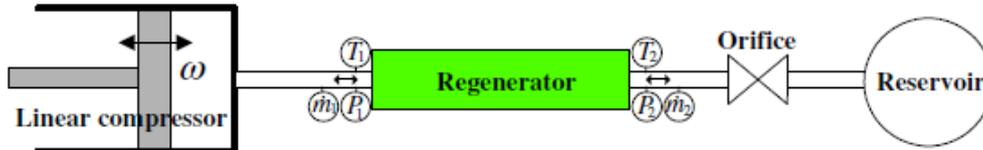
Fig 1: Schematic diagram of experimental apparatus
